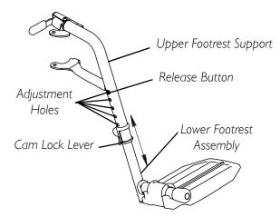
FIGURE 6.2 Adjusting the Footrest Height
